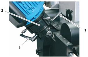
Remove both clamping levers (1) on the upper and lower side of the milling unit.
