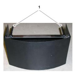
Insert both pins (1) into the holes on the underneath of the milling unit.
