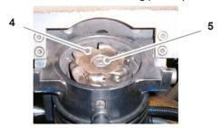
Remove the fastening screws (5) and remove the milling head (4).
